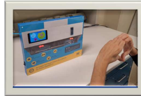
TOF Based Hand Gesture Recognition on STM32F4
